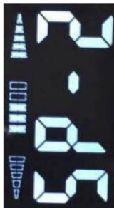
Turn **Function Wheel** left and right to select Delay time setting, turn **Parameter Knob** right or left among 0.2-2.0 seconds (DL-0.2-2.0) to adjust and press for confirm.
