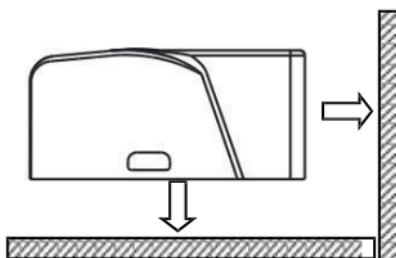
Step2 : Insert the stander charging port contact the stander. Connecting USB cable.
