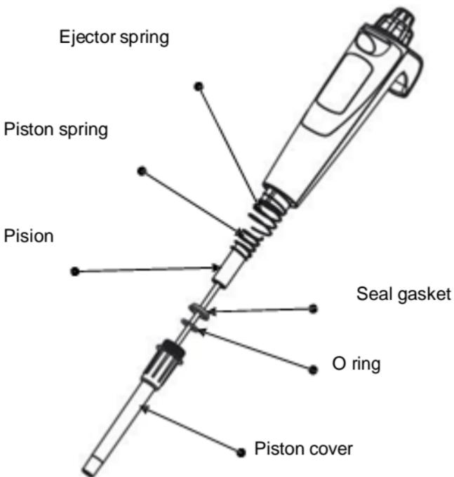
**Note!** The unidentified parts can never be autoclaved or disassembled prior to authorization.
